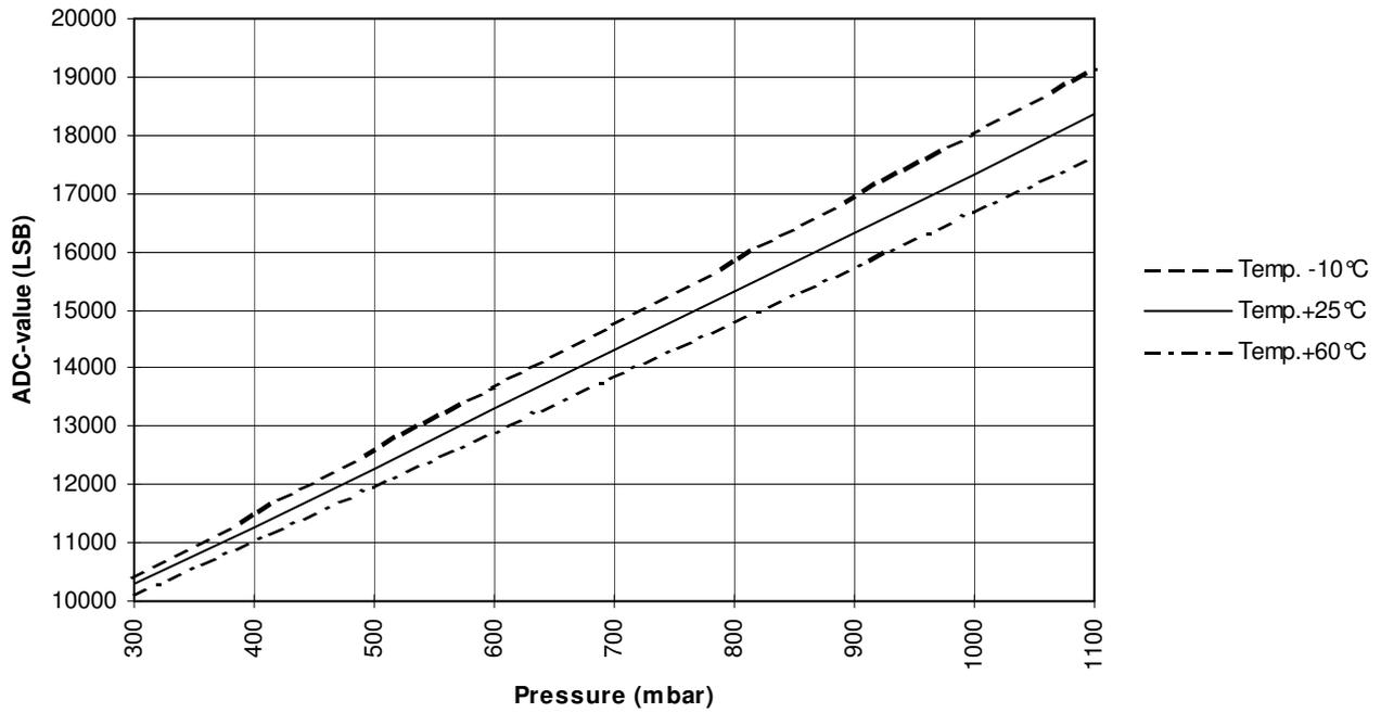
**ADC-value D2 vs Temperature (typical)**
