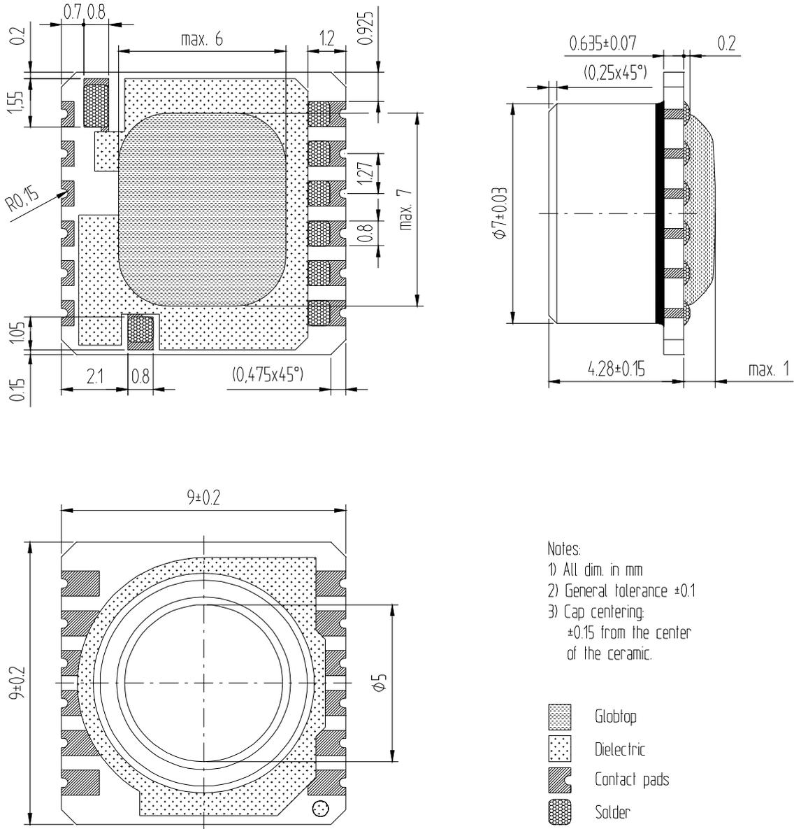
Fig. 9: Device package outlines of **MS5534AM (RoHS)**.
