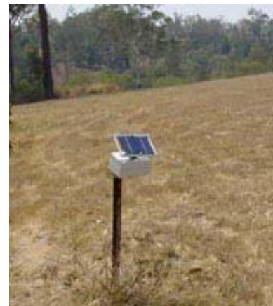
Solar powered environmental measurement station based on Fleck technology.
